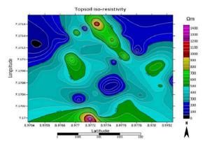
Fig. 8 Iso-resistivity map for layer one.
