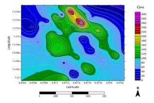
Fig. 9 ISO-resistivity map for the second layer.
