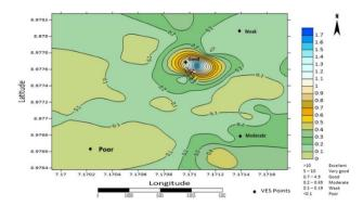
Fig. 7 Longitudinal conductance variations of the study area
