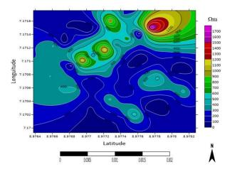
Fig. 10 Iso-resistivity of the third layer.
