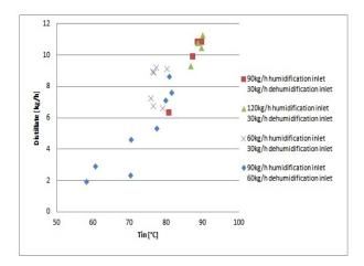
Fig. 3. Amount of water produced as function of feed water temperature at inlet of the humidification for different water flow rates at both the dehumidification and humidification chamber inlets
