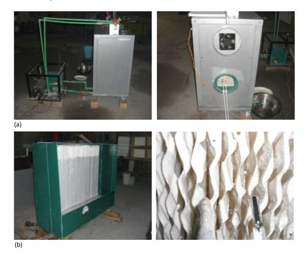
Fig 1(a): Side view of the desalination unit Fig. 1(b): view of the inner core (membrane) of the desalination system showing fresh water condensation
