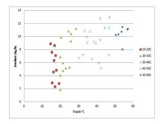
Fig. 5: Amount of fresh water produced as function of temperature at the inlet of the dehumidification chamber.
