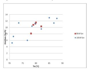
Fig. 4. Amount of fresh water produced as function of temperature at the inlet of the humidification chamber for two different air mass flow rates
