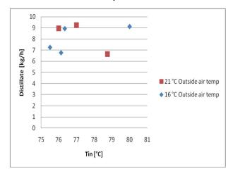
Fig. 6: Amount of water produced as function of temperature at inlet of the humidification chamber for two different weather conditions
