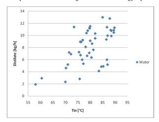
Fig. 7: Amount of fresh water produced as function of temperature at inlet of the humidification chamber.
