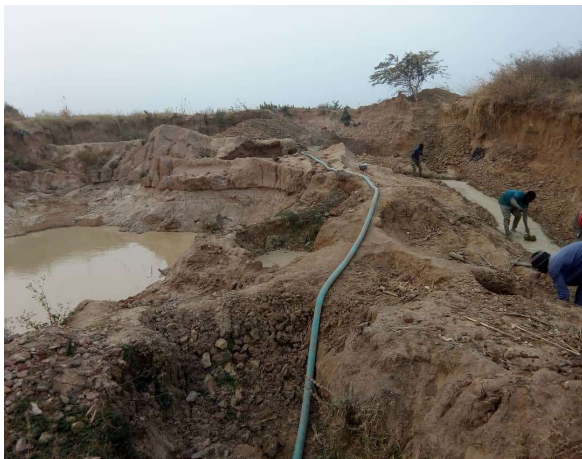
Fig. 1 Local Separation of the Cassiterite from the gravel sand
