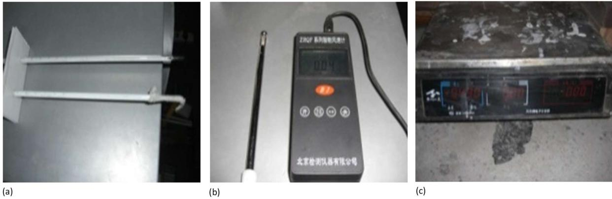
Fig. 2. (L-R) Dry/Wet bulb thermometer (a) Air flow meter (b) Scale (c)
