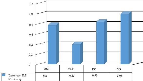
Fig. 2. Unit water cost comparison of major desalination technologies
