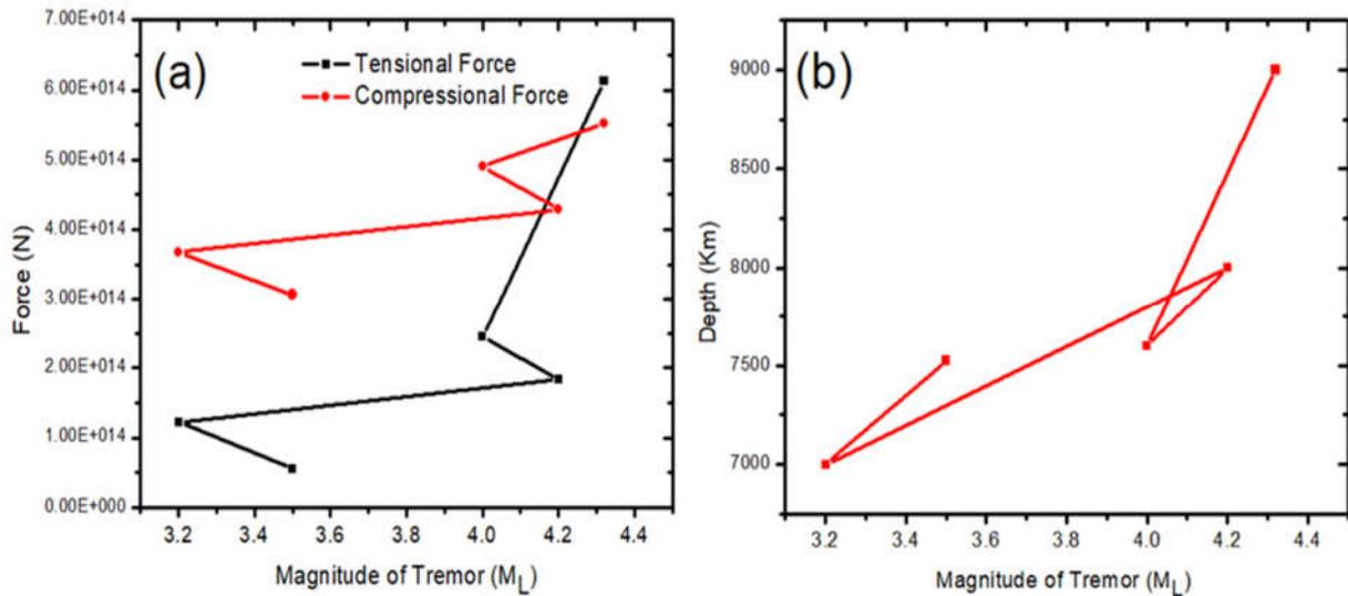
Fig. 15 Variation of Depth and Force with the Magnitude of Tremor
