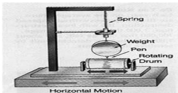
Fig. 8 Features of the Seismograph or Seismometer
