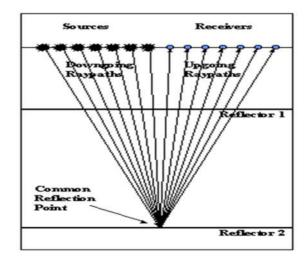
Fig. 11 Common Depth Point Reflection method
