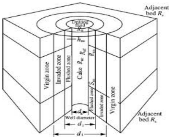
Fig. 5 Cross Section of a Well Bore, Penetrating a Permeable Formation [29].
