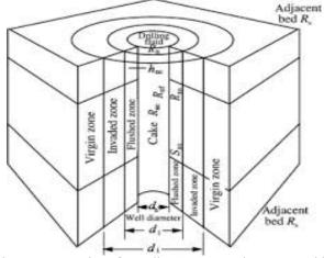
Fig. 5 Cross Section of a Well Bore, Penetrating a Permeable Formation [29].
