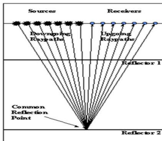
Fig. 11 Common Depth Point Reflection method
